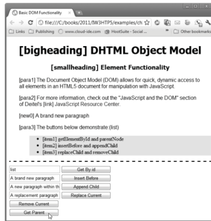
Fig. 12.11 | The document of Figure 12.4 after using the Get By id button to item2 , then using the Get Parent button to select item2 's parent—the unordered list.
