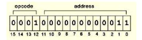
• We see that the opcode is 1 and the address from which to load the data is 00000000011
