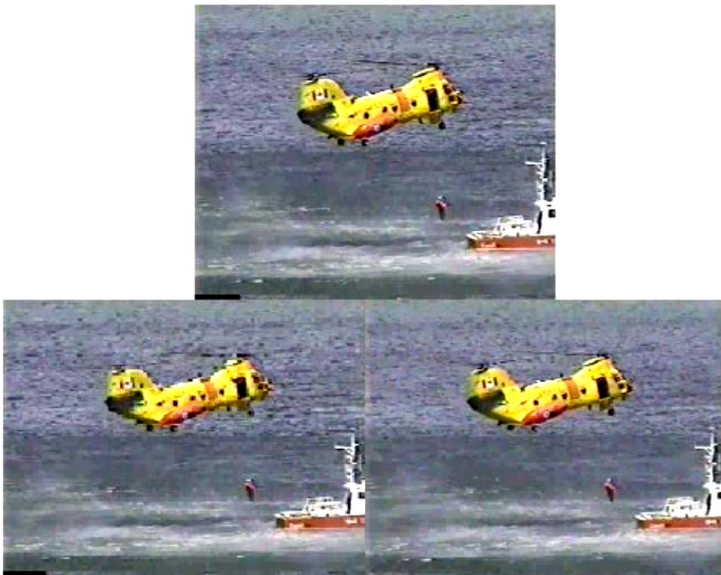
Fig. 1: Interlaced scan produces two fields for each frame. At top: The video frame, at left: odd field, at right: even field,
