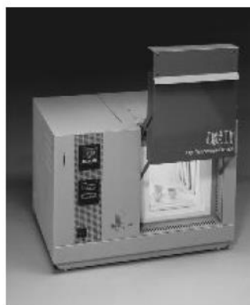
Example of a muffle furnace used for heating samples to maximum temperatures of 1100–1700 °C.
