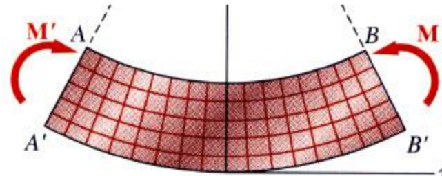
Beam after bending
