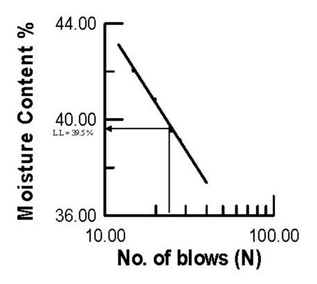
The soil is heavily preconsolidated since  $\omega_n$  is smaller than P.L & lower than L.L.
