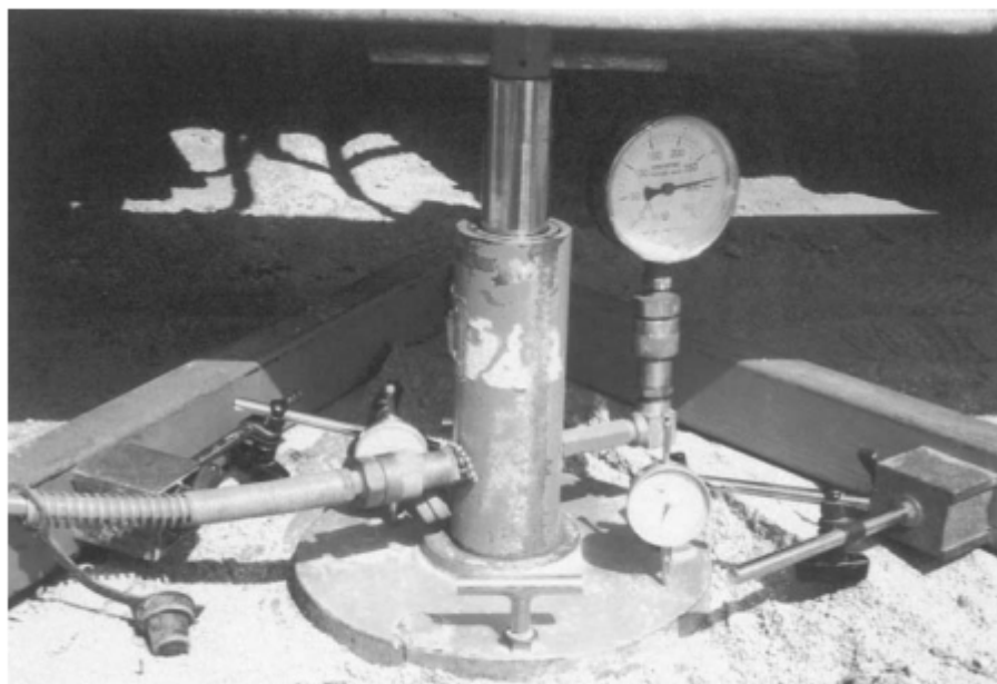
Figure 4.26 Plate load test in the field (Courtesy of Braja M. Das, Henderson, Nevada)
