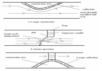
After construction is complete the 2-stage the cofferdam is removed and flow is diverted through the part of the dam (spillway or powerhouse).
