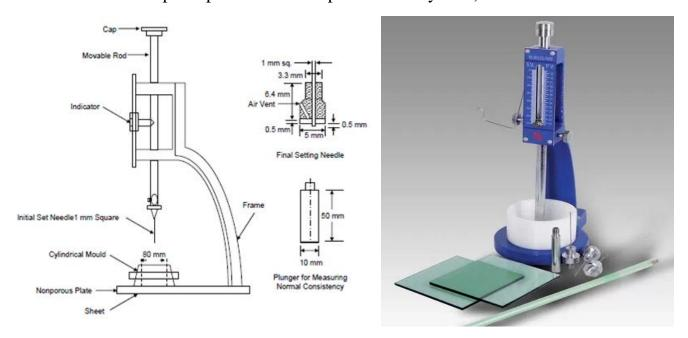
Vicate instrument for standard consistence and setting of cement
