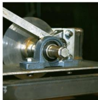
This journal bearing supports the end of the shaft. (5)
