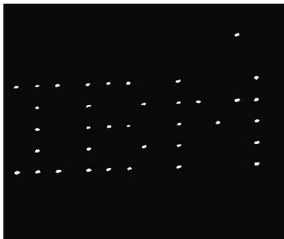
Fig. 2.32. Manipulation of single Xe atoms on a Ni(110) surface with an atomic force microscope (with kind permission of Dr. Eigler)
