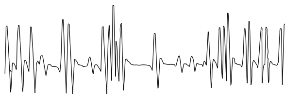
Fig. 11.63. Derivative saturation spectrum of the iodine transition B^3\Pi_u (v' = 58, J' = 99) \leftarrow X^1\Sigma_g^+ (v'' = 1, J'' = 98) with 21 hfs components
