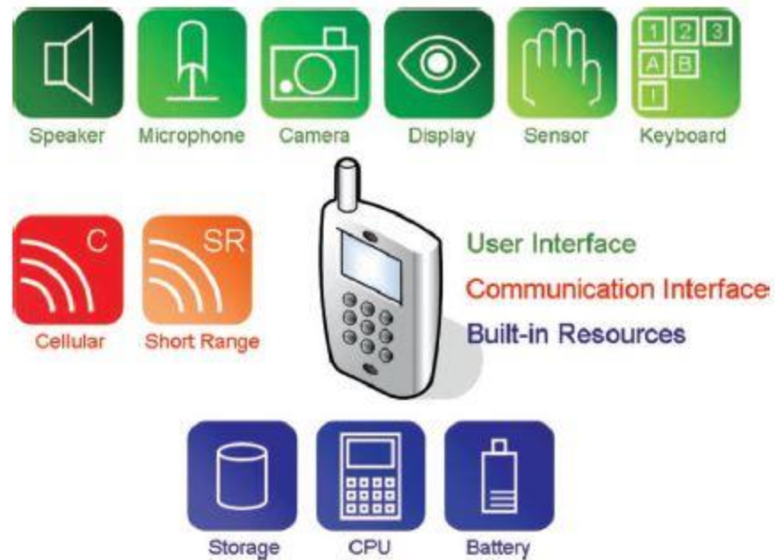
Figure 1.4. A mobile device broken up into the several capabilities grouped into the user interface, communication interface, and the built-in resources.
