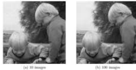
Figure (6): Image averaging to remove Gaussian noise.
