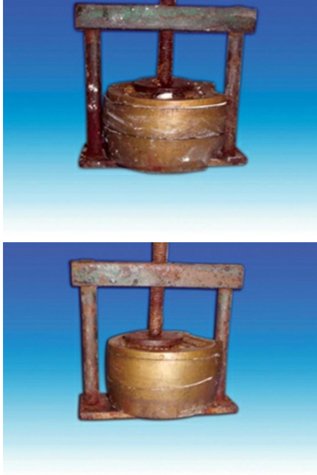
FIG 3.4.8.16 Completed flask ready for dewaxing
