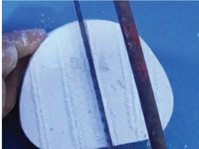
FIG 3.4.9.4 Removal of stone using saw blades
