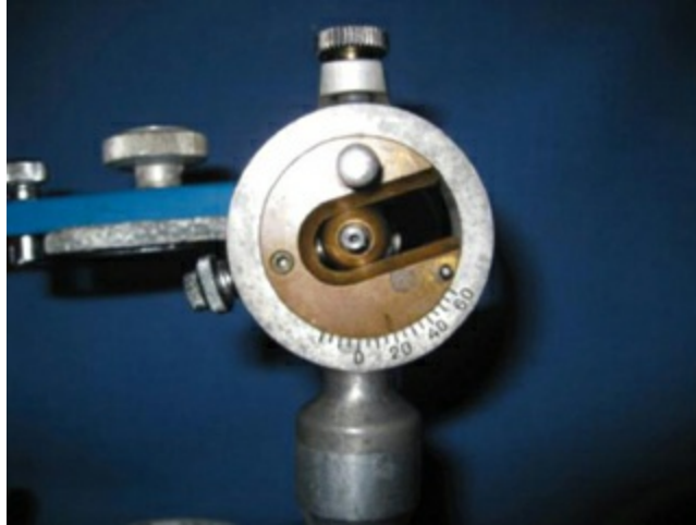
FIG 1.1.8.4 Condylar sphere in the upper member and condylar track in the lower member
