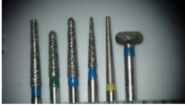
FIG 2.1.28 Diamond abrasive points
