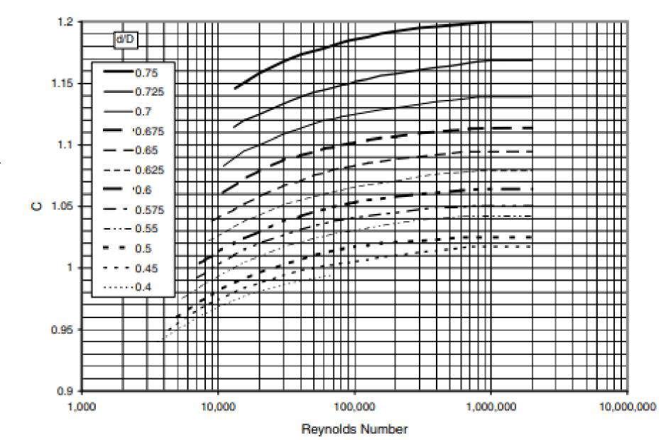
Choke flow coefficient for orifice-type chokes.
