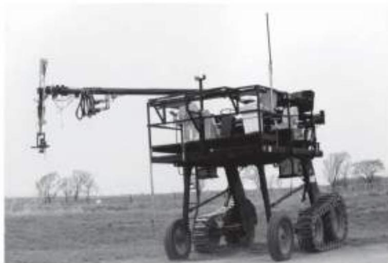
**Figure 4:** All-terrain instrument platform designed for collecting spectral measurements in agricultural cropland environments. (Courtesy of the University of Nebraska-Lincoln Center for Advanced Land Management Information Technologies.)
