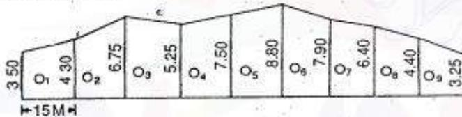
**Example:** A tract of land has three straight boundaries AB, BC, and CD. The fourth Boundary DA is irregular. The measured length are as under
