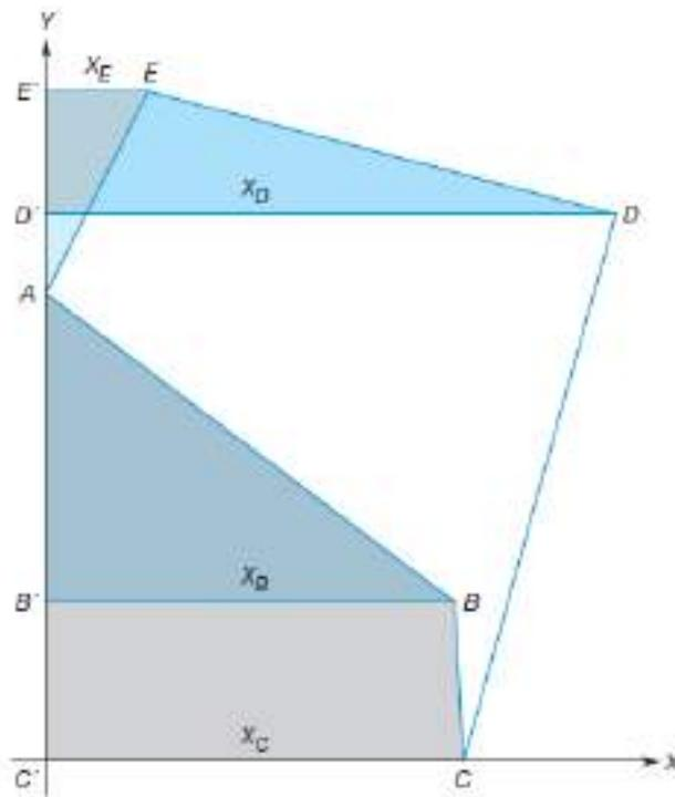
As shown in that figure, it is convenient (but not necessary) to adopt a reference coordinate system with the X and Y axes passing through the most southerly and the most westerly traverse stations, respectively.
