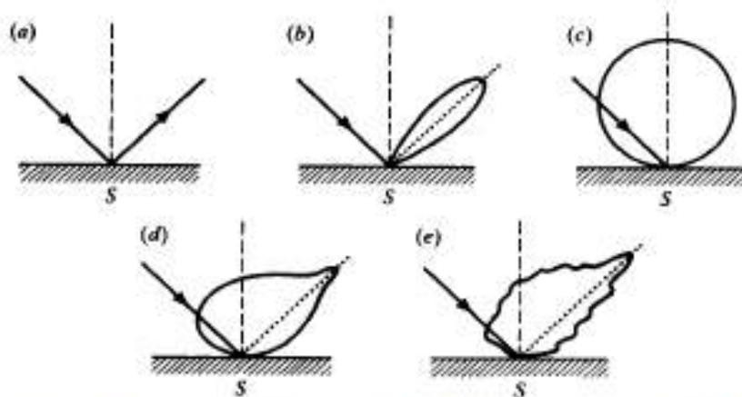
Figure 4. Different types of scattering surfaces (a) Perfect specular reflector (b) Near perfect specular reflector (c) Lambertian (d) Quasi-Lambertian (e) Complex.
