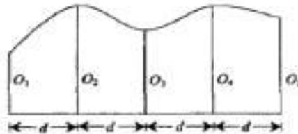
The area of each trapezoid is determined and added together to derive the whole area. If there are  $n$  offsets at equal interval of  $d$  then the total area is
