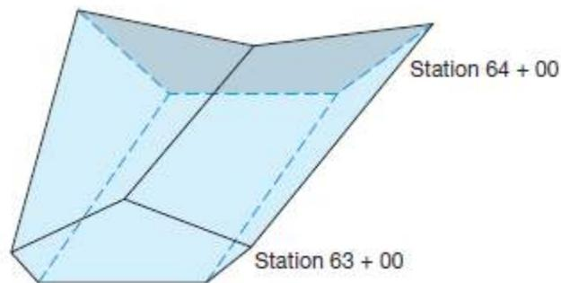
However, from a practical standpoint, the differences in volumes computed by the average-end-area method and the prismoidal formula are usually so small as to be negligible. Where extreme accuracy is needed, such as in expensive rock cuts, the prismoidal method can be used. One arrangement of the prismoidal formula is:
