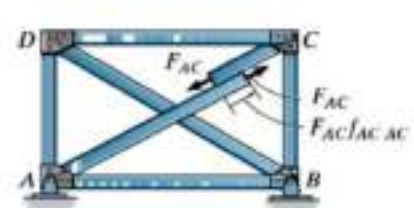
redundant F_{AC} applied
