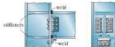
typical "fixed-supported" connection (metal) (b)
