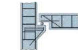
typical "roller supported" connection (concrete) (a)
