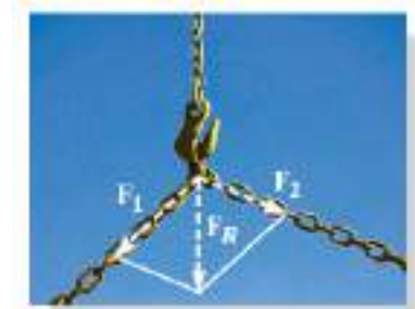
The parallelogram law must be used to determine the resultant of the two forces acting on the hook.
