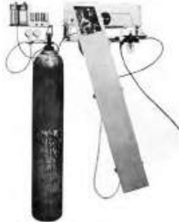
Fig. 4.6 Bubble Gauge—Stevens Manometer Servo (Courtesy: Leupold and Stevens, Inc. Beaverton, Oregon, USA)
