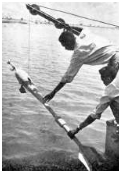
Fig. 4.10 Propeller-type Current Meter—Neyrtec Type with Sounding Weight
