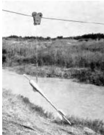
Fig. 4.12(b) Neyrtec Type Meter in a Cableway
