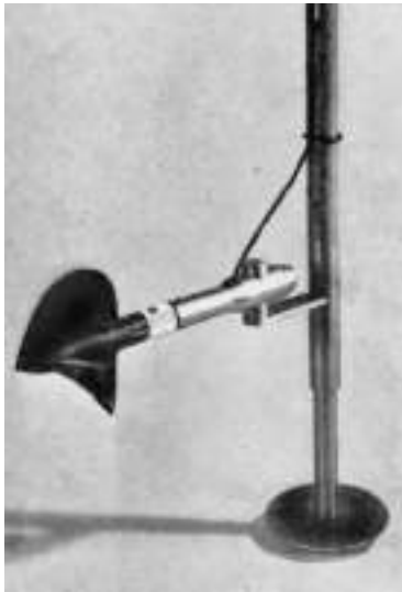
Fig. 4.12(a) Neyrtec Type Current Meter for use in Wading (Courtesy: Neyrtec, Grenoble, France)
