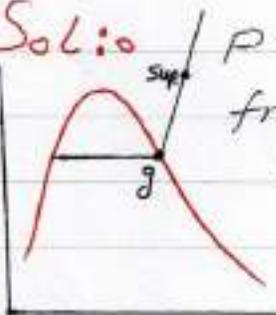
from Charles's law  $\frac{v_g}{T_{\text{sat}}} = \frac{v_{\text{sup}}}{T_{\text{sup}}}$  (for 1 kg)
