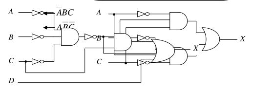
The expression for the output of the circuit is:  $X = (\overline{A}\overline{B}\overline{C})C + \overline{A}\overline{B}\overline{C} + D$
