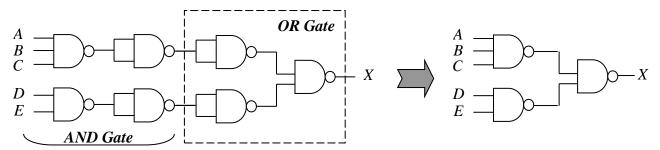
**Example:** Implement the logic circuit that has the expression  $X = \overline{AB.(\overline{C+D})}$  using only one NAND and NOR gate.
