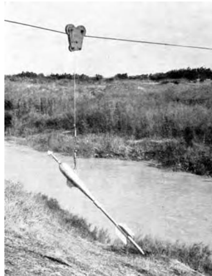
Fig. 4.12(b) Neyrtec Type Meter in a Cableway
