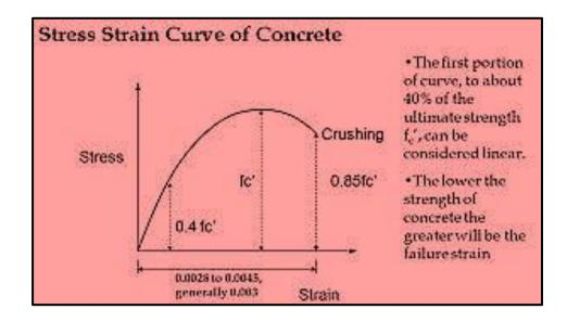
3- Modulus of Elasticity for Concrete: Modulus of Elasticity of Concrete can be defined as the slope of the line drawn from a stress of zero to a compressive stress of 0.45f'c. As concrete is a heterogeneous material. The strength of concrete is dependent on the relative proportion and modulus of elasticity of the aggregate.
