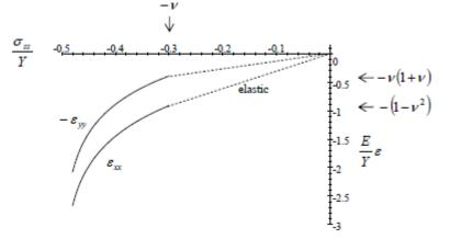
through the plastic compression; the plastic strains are of comparable size to the elastic strains. There is a rapid change of stress and then little change once  $\sigma_{zz}$  has approached close to its limiting value of – Y/2.
