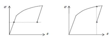
cases), since there is no unique relationship between the current stress and the current strain. However, one can relate the current stress to the current **increment in strain**, and these are the "stress-strain" laws which are used in plasticity theory. The total strain can be obtained by summing up, or integrating, the strain increments.
