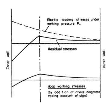
show that the maximum tensile stress, instead of being at the bore as in the plain cylinder, is now at the elastic/plastic interface position.
