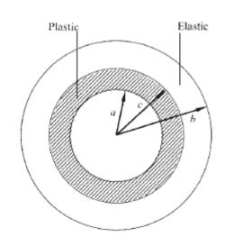
At  $r = c^-$ , i.e. in the plastic area, the radial stress is determined by eqn.(1):
