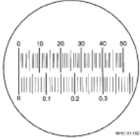
Fig. 3.26 Calibration of an ocular micrometer with a stage micrometer
