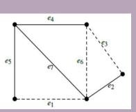
$$B_{f} = \begin{bmatrix} 0 & 1 & 1 & 1 & 0 & 0 & 1 \\ 0 & 0 & 0 & 1 & 0 & 1 & 1 \\ 1 & 0 & 0 & 0 & 1 & 0 & 1 \end{bmatrix} \sim \begin{bmatrix} 1 & 0 & 0 & \vdots & 1 & 1 & 0 & 1 \\ 0 & 1 & 0 & \vdots & 0 & 1 & 0 & 1 \\ 0 & 0 & 1 & \vdots & 0 & 0 & 1 & 1 \end{bmatrix}$$
