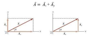
From the figure and the definition of sine and cosine, we see that  $(\cos \theta = A_x / A)$  and that  $(\sin \theta = A_y / A)$ . Hence, the components of  $\vec{A}$  $A_x = A \cos \theta$  and  $A_y = A \sin \theta$
