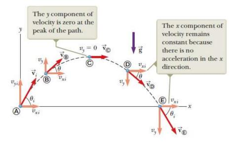
When analyzing projectile motion, model it to be the superposition of two motions: (1) motion of a particle under constant velocity in the horizontal direction and (2) motion of a particle under constant acceleration (free fall) in the vertical direction.
