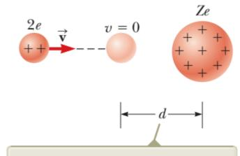
Because of the Coulomb repulsion between the charges of the same sign, the alpha particle approaches to a distance *d* from the nucleus, called the distance of closest approach.
