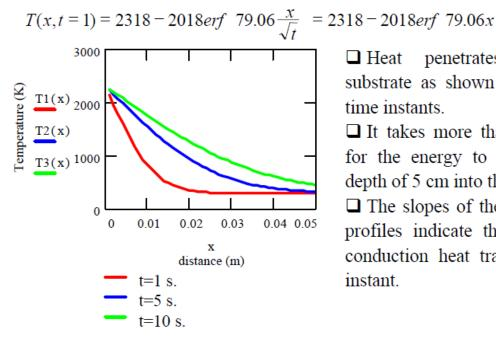
Heat penetrates into the substrate as shown for different time instants.
