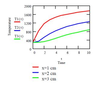
□ At x=1 cm, the temperature rises almost instantaneously at a very fast rate. A short time later, the rate of temp. increase slows down significantly since the energy has to distribute to a very large mass.
