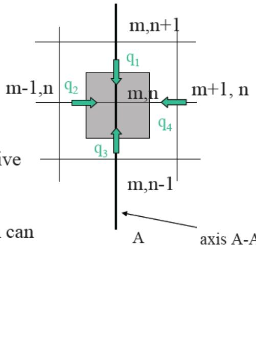
□ Insulated surface case: If the axis A-A is an insulated wall, therefore there is no heat transfer across A-A. Also, the surface area for  $q_1$  and  $q_3$  is only half of their original value.
