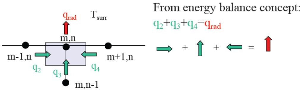
$$k \left( \frac{\Delta y}{2} \right) \frac{T_{m-1,n} - T_{m,n}}{\Delta x} + k (\Delta x) \frac{T_{m,n-1} - T_{m,n}}{\Delta y} + k \left( \frac{\Delta y}{2} \right) \frac{T_{m+1,n} - T_{m,n}}{\Delta x} = \varepsilon \sigma (\Delta x) (T_{m,n}^4 - T_{\text{surr}}^4)$$
