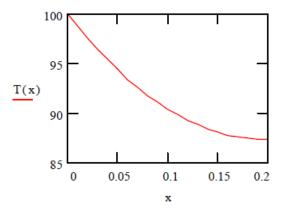
As shown, temperature drops off very quickly. At the midpoint T(0.1)=90.4°C. At the end T(0.2)=87.3°C.
