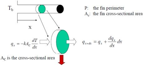
$dq_{conv} = h(dA_s)(T - T_{\infty})$ , where  $dA_s$  is the surface area of the element
