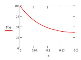
Temperature at the handle (x=0.2 m) is only 37.3 °C, not hot at all. This example illustrates the important role played by the thermal conductivity of the material in terms of conductive heat transfer.
