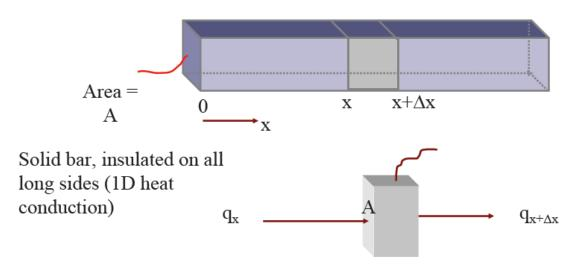
$\dot{q}$  = Internal heat generation per unit vol. (W/m<sup>3</sup>)
