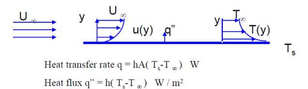
h=heat transfer co-efficient (W /m2K)
