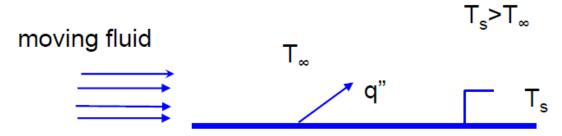
❖ Energy transferred by diffusion + bulk motion of fluid
