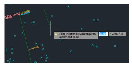
Note that there is a difference between the angle defined by the software and the bearing definition as shown in the figure below
