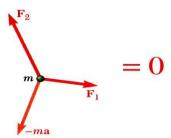
If we include inertia vector, the system of forces acting on particle is equivalent to zero. The particle is said to be in dynamic equilibrium.
