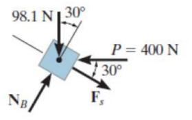
**Spring Force F<sub>s</sub>.** In the initial position the spring is stretched  $s_1 = 0.5$  m and in the final position it is stretched  $s_2 = 0.5$  m + 2 m = 2.5 m. We require the work to be negative since the force and displacement are opposite to each other. The work of  $\mathbf{F}_s$  is thus
