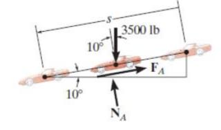
**NOTE:** If this problem is solved by using the equation of motion, *two steps* are involved. First, from the free-body diagram, Fig. , the equation of motion is applied along the incline. This yields
