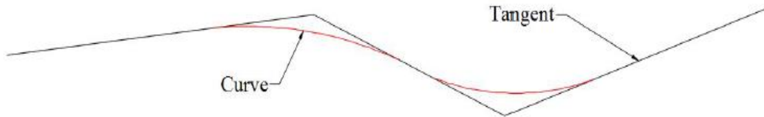
a: Two-dimensional horizontal curve
