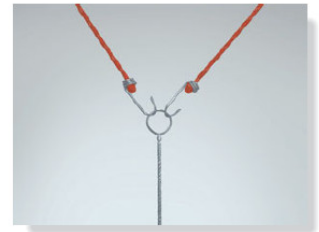
Three forces act on the ring. Since these forces all meet at point, then for any force analysis, we can assume the ring to be represented as a particle.
