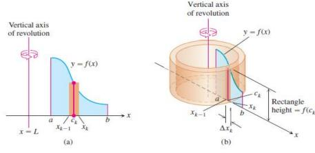
$$V = \int_{a}^{b} 2\pi (\text{shell radius})(\text{shell height}) dx.$$
