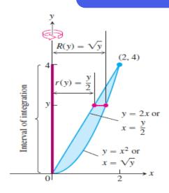
The region bounded by the parabola  $y = x^2$  and the line y = 2x in the first quadrant is revolved about the y-axis to generate a solid. Find the volume of the solid.
