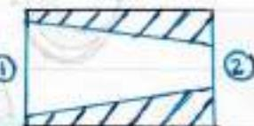
$$\therefore h_2 = h_1 + \frac{1}{2} (C_1^2 - C_2^2) * 10^3$$
