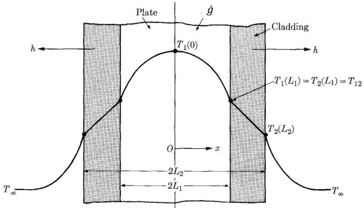
Figure 2.4: The fuel element of a pool reactor.
