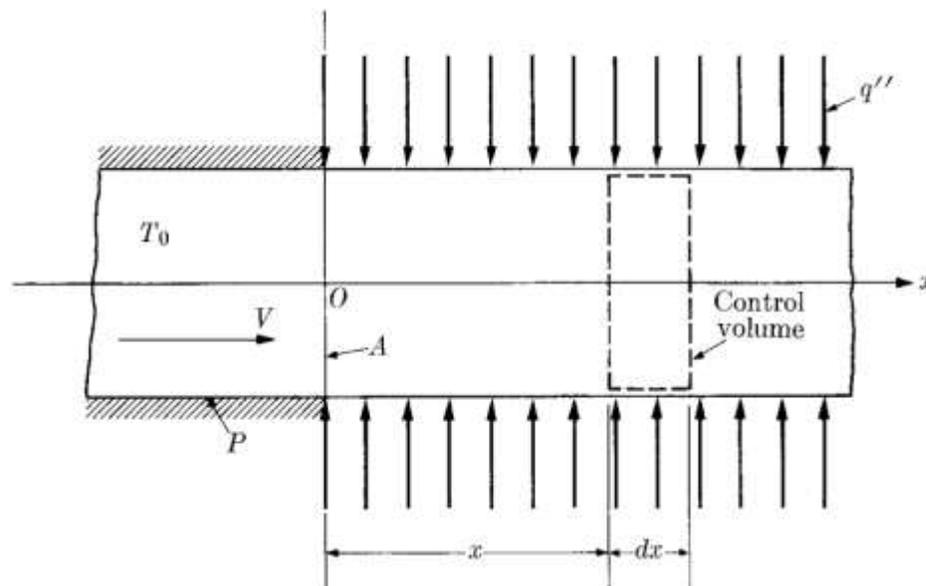
Consider the radially lumped, axially differential control volume shown in Figure 2.5. Let us apply the general laws to this control volume as follows.
