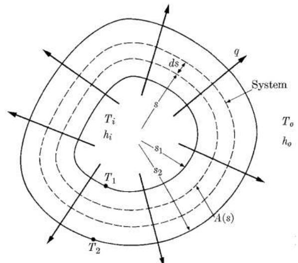
**Figure 2.1:** a long, hollow cylinder or a thick-walled, closed shell of constant wall thickness.
