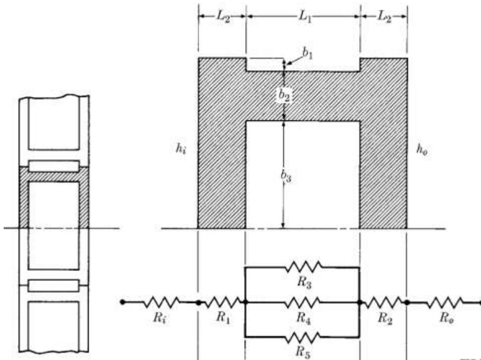
**Figure 2.3:** A wall composed of hollow concrete blocks.
