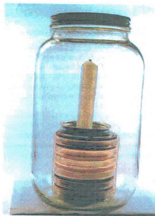
FIGURE 4.9 A candle jar. The candle is lit just before sealing the jar. As the candle burns, it consumes oxygen and produces carbon dioxide. When most of the oxygen in the jar is used up, the flame goes out.
