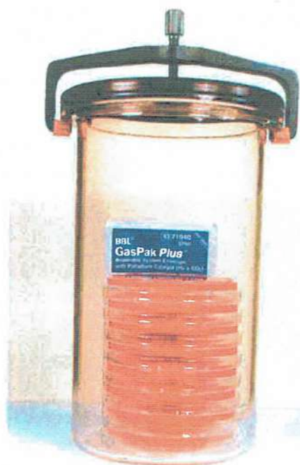
FIGURE 4.11 An anaerobic jar. The contents of the GasPak Plus™ envelope, when activated by water, consume oxygen and produce an atmosphere of hydrogen and carbon dioxide.
