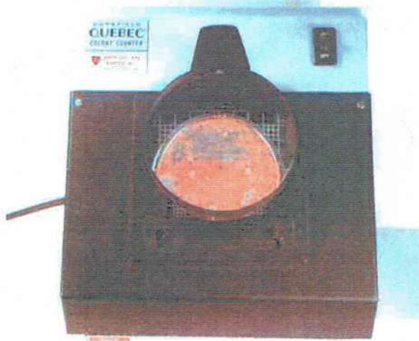
FIGURE 4.49 A colony counter. The magnification it provides can aid in the selection of colonies from agar plates.
