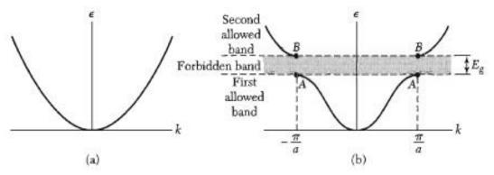
We explain physically the origin of energy gaps in the simple problem of a linear solid of lattice constant a. The low energy portions of the band structure are shown qualitatively, in figure (a) for entirely free electrons and in figure (b) for electrons that are nearly free, but with an energy gap at  $k = \pm \pi/a$ . The Bragg condition  $(k + G)^2 = k^2$  for diffraction of a wave of
