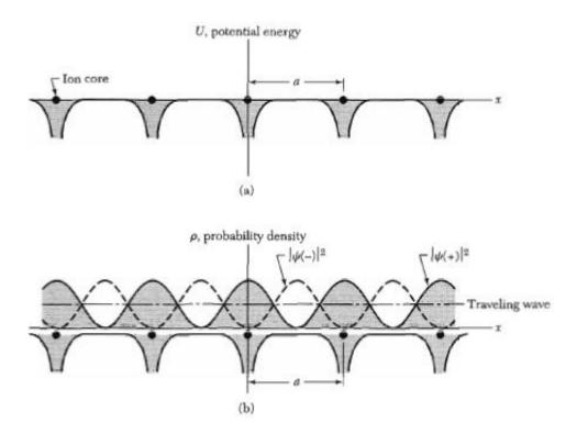
Figure (a) the variation of the potential energy of a conduction electron in the field of the positive ion cores.
