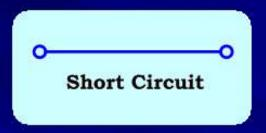
The current through a short circuit is generally not equal to zero. However, the voltage across a short circuit is always equal to zero, because:
