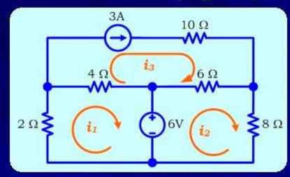
Solution: Mesh 1 & 2 does not contain current sources.
