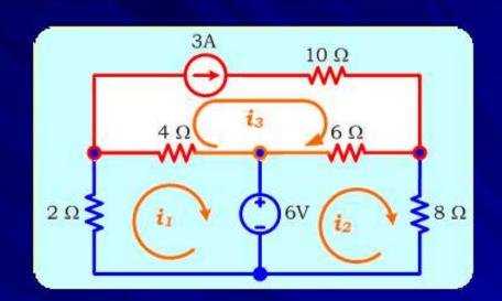
Mesh 3 contains a 3A current source (not shared by another mesh) Do not apply KVL (because KVL involves voltage across the current source).
