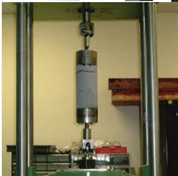
Figure 2.3-10: Samples of concrete direct tension specimen (2).
