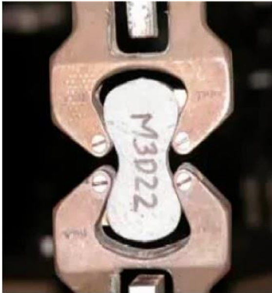
Figure 2.3-11: Samples of concrete direct tension specimen (3).
