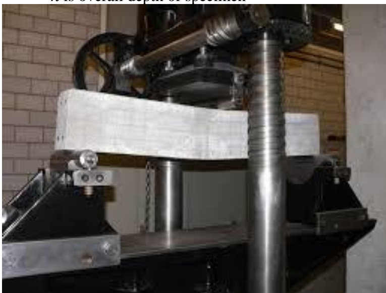
Figure 2.3-12: Modulus of rupture for concrete tensile strength.
